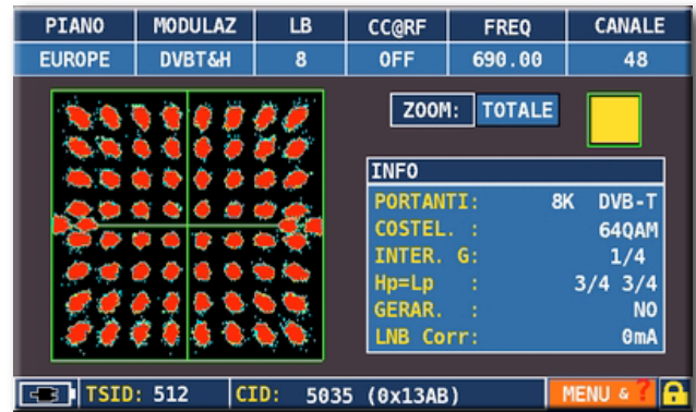
Figure 2: Example with DVB-T signal constellation (64QAM) detected after 60 seconds of measurement. Note that because of the high presence of residual AC, the constellation explodes from the center to outwards, the halos of the constellation become elliptical rather than circular.
