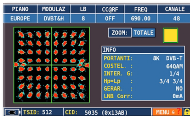
Figure 5: Constellation DVB-T signal (64QAM) detected after 15 seconds of measurement (with high presence of residual AC)
