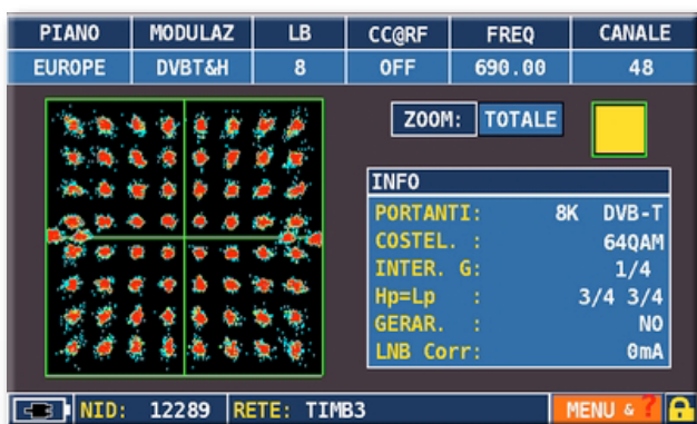
Figure 4: Constellation DVB-T (64QAM) detected after 5 seconds of measurement (with high presence of residual AC)
