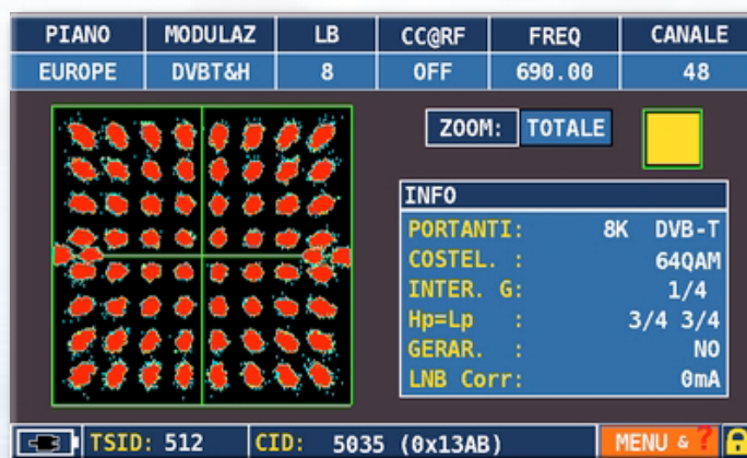
Figure 6: Constellation DVB-T (64QAM) detected after 60 seconds of measurement (with high presence of residual AC)
