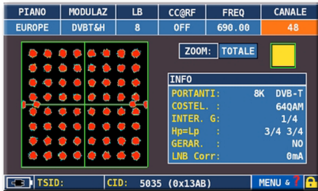
Figure 1: Example DVB-T signal constellation (64QAM) detected after 60 seconds of measurement (no presence of residual AC). Note that the halos are all perfectly circular.
