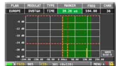
ECHO MEASUREMENT in SFN networks, with impulse response in real time, green area shows the guard interval
