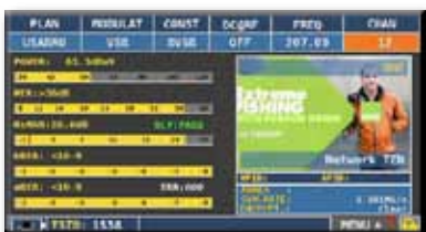
VSB signal, all the measurements, picture and settings on one screen
