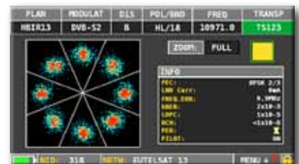
DVB-S2 multistream Constellation 8PSK mod., on the right relative modulation parameters & ISSY
