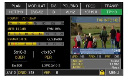
Fig. 10 when measuring in SCR mode, the user band shows on the bottom left side of the screen
