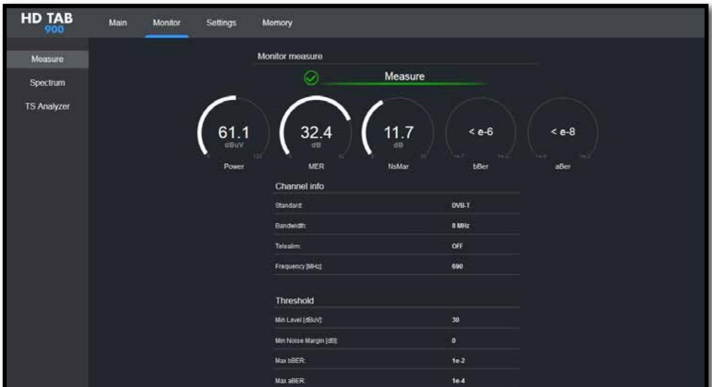
Example of MEASUREMENTS of a TV CHANNEL (DVB-T Standard) and related screen of IMPULSE RESPONSE (ECHOES)
