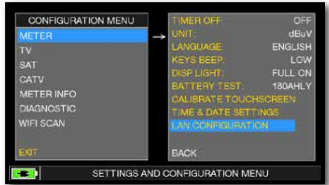
Touch "METER" and then "LAN CONFIGURATION"
