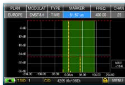
Fig. 2: GOOD RECEPTION:* 2 ECHOES present, but within the guard interval mask (green area) coming from a distance of: 1st echo: 24,50 Km, the same as a 81,67 \mu s delay.
