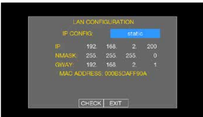
Touch "IP CONFIG" and select "STATIC", insert the "IP", "NMASK" and "GWAY" parameters.
