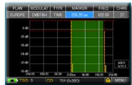
Fig. 3: MARGINAL RECEPTION (or IMPOSSIBLE):* 2 ECHOES present outside the guard interval mask (green area), coming from a distance of: 1st echo: 70,56 Km, the same as a 235,20 \mu s delay.
