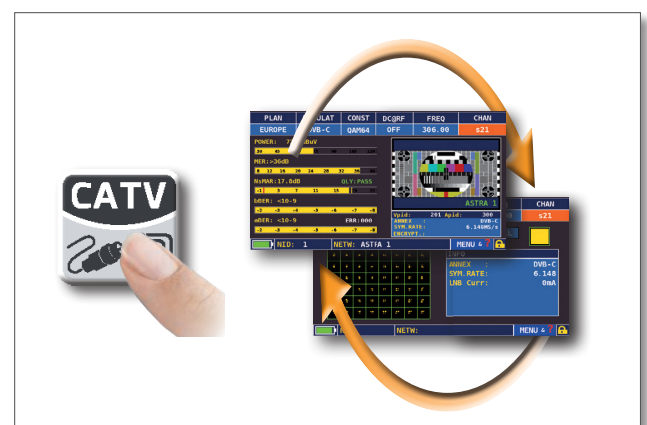
Press repeatedly to navigate in the CATV measurement screens
