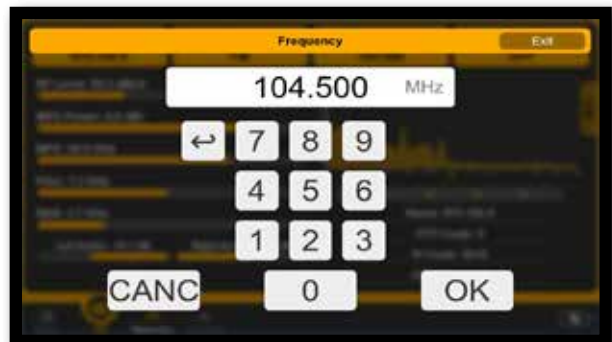
Touch FREQUENCY if you want to change the frequency received
