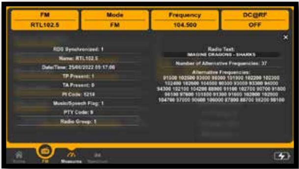
RDS transmission parameters list example
