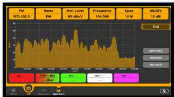
Touch MARKERS to access to the MARKERS SETUP MENU
