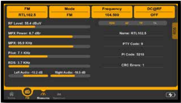
FM transmission parameters list example
