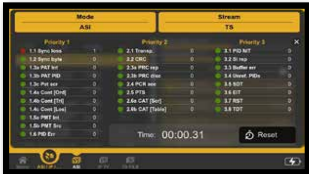
Touch ETR-290 ICON to start ETR-290 analyzer
