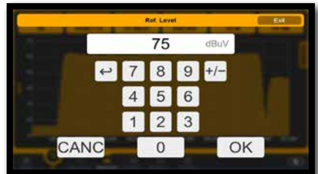
Touch REFERENCE LEVEL to change the Reference Level value
