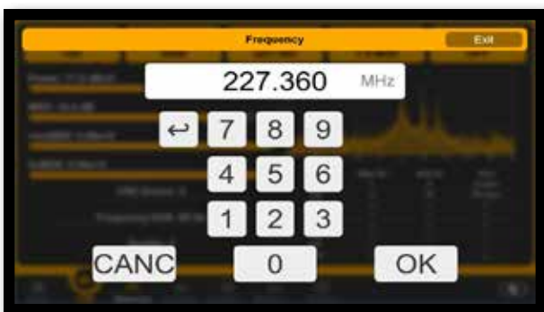
Touch FREQUENCY if you want to change the Frequency received
