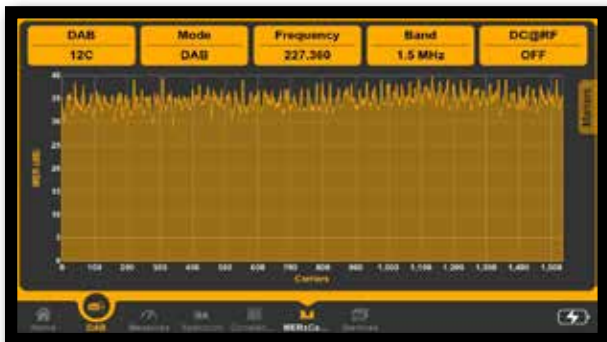
DAB MER VS CARRIER analyser example
