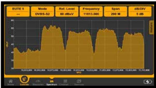
5 dB div SAT Spectrum example
